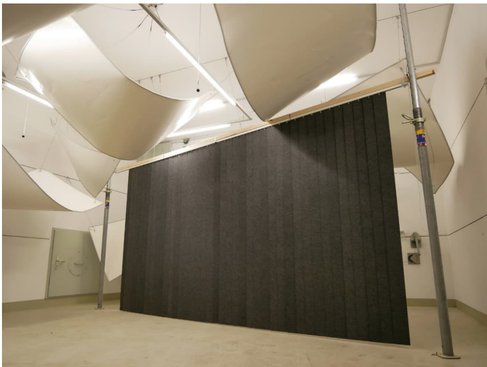
Figure B.6. Test object mounted in the reverberation room, opening angle 0^\circ – closed, hanging freely in the reverberation room.
