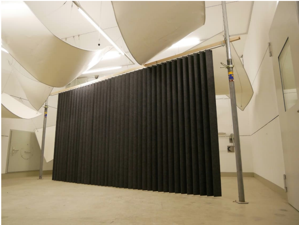
Figure B.5. Test object mounted in the reverberation room, opening angle 45^\circ – semi-open, hanging freely in the reverberation room.
