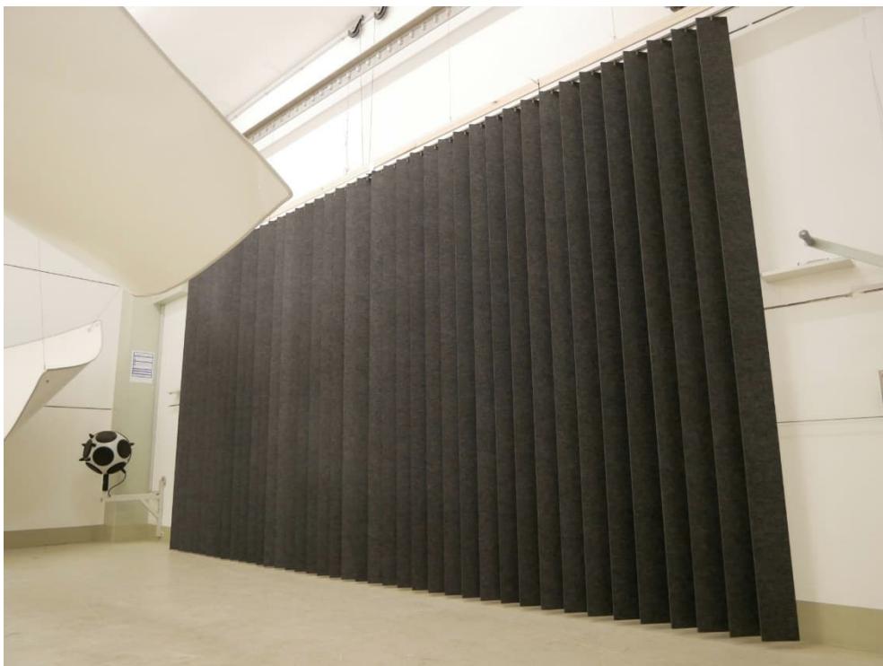
Figure B.2. Test object mounted in the reverberation room, opening angle 45° – semi-open, 150 mm distance to the wall.
